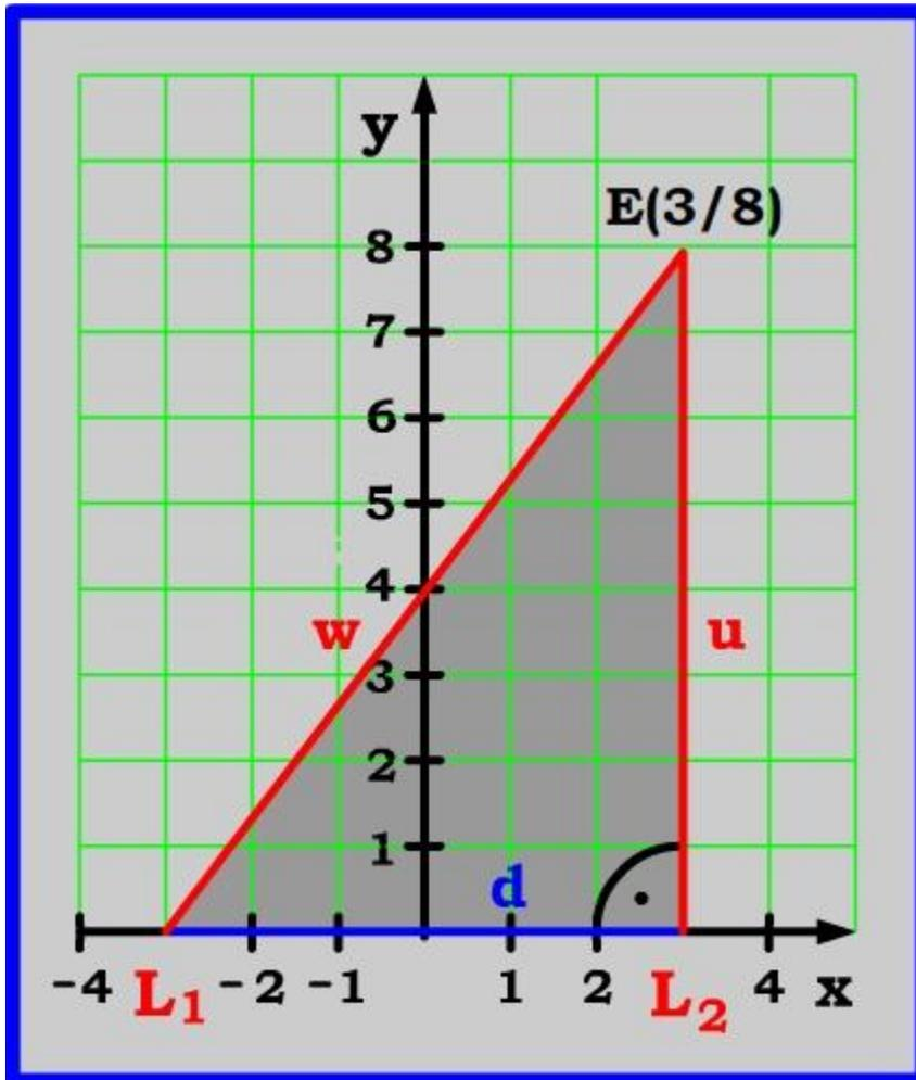
$$\mathbf{b)} \quad w = \sqrt{d^2 + u^2} = \sqrt{(6 \text{ m})^2 + (8 \text{ m})^2} = \sqrt{100 \text{ m}^2} = 10 \text{ m}$$
