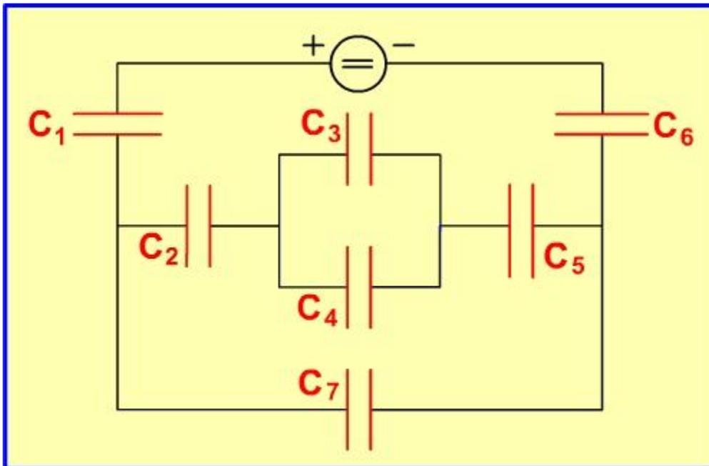
$$C_1 = 8 \mu\text{F}, \quad C_2 = 3 \mu\text{F}, \quad C_3 = 12 \mu\text{F}, \quad C_4 = 6 \mu\text{F}$$
